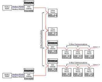
In this configuration the DSX Gateway is configured as a Network Level 2 gateway using DIP SW1.3 and SW1.4. The address mapping results in the same Modbus address mapping as defined in the Network Level 1 section.
