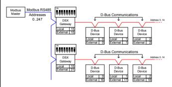
If 3<sup>rd</sup> party Modbus devices are added to the External Modbus network the addressing of these devices and the DSX Gateways must be configured so that there are no address clashes. The baud rate and parity must also be configured the same on all devices.
