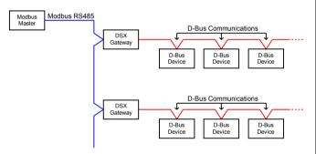
Each DSX Gateway performs *Address Mapping* to allow a single Modbus Master to uniquely address the devices on different D-Bus networks.
